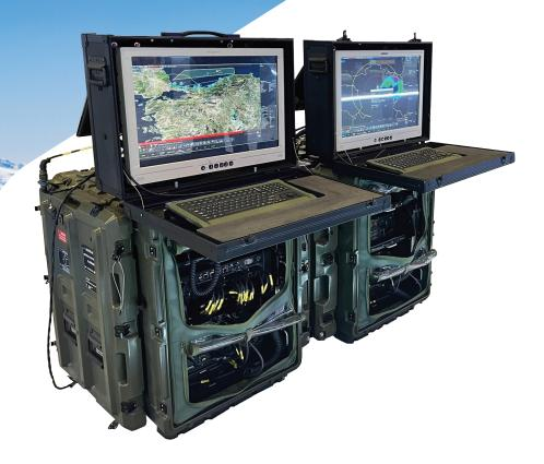
Deployable Air Defense Operation Center (HERİKKS 600-T) is an air defense early warning and command, control, communications, computers and intelligence (C4I) system that manages the air defence activities on tactical level. HERİKKS 600-T can be used as a backbone system for all air defense sensors and effectors in the tactical field, and serve as the main command and control system in the air defense activities of a particular point (base, port, critical facilities, etc.).
