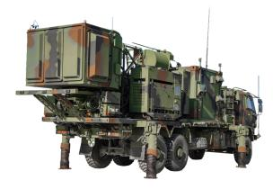
Radar EA System has the capability of suppressing threat radar coverage or disabling radar functions for desired durations by applying various jamming and deception electronic attack techniques. System can identify threat radars within the mission zone by its 'Support Measure Infrastructure'. With its DRFM based structure, system can apply coherent and non-coherent jamming/deception techniques against threat radars.
