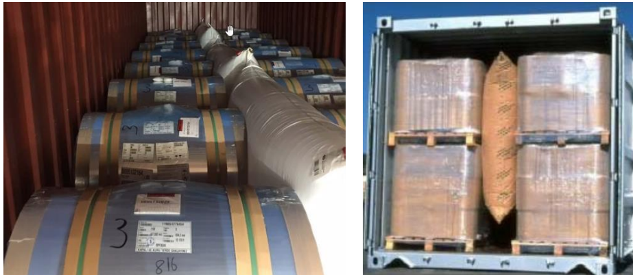
Figure-35: In-Container Load Blocking:
