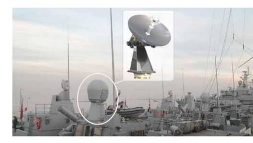
Stabilized Satellite Communication Terminals, which provide reliable and uninterrupted communications on the move on airborne, naval and land platforms, are designed and manufactured to be light and compact and in accordance with military standards. With the Manpack, Flyaway, SATCOM On The Pause and SATCOM On The Move Satellite Communication Terminals within the ASELSAN product family, solutions are offered which meet the communications needs of land platforms.
